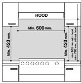
e) The dimensions of the cutout for the appliance must be those indicated in the figure D. Clamps are provided to fasten the hob to counters measuring from 20 to 40 mm in thickness. To fasten the hob securely, it is recommended that all the clamps be used.
